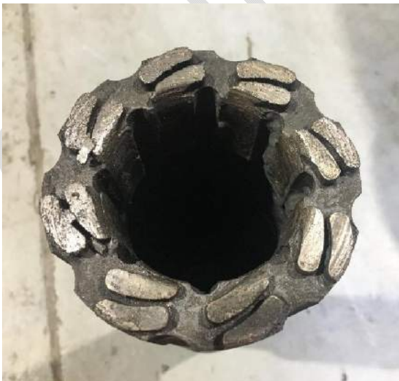
Figure 15 - Mill bit following milling of Owen Oil Tools Magna Plug
