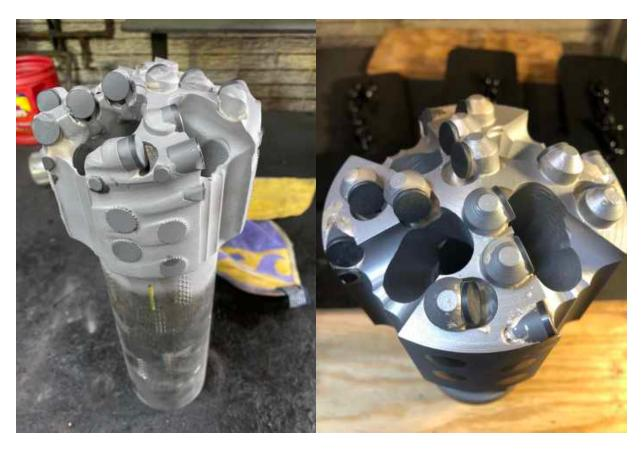
Stick Pipe reverse circulation 8,120 ft of abrasive fill and scale in 53 hours. In gage and refit with two new cutters.
