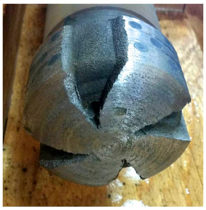
Test was done with 780 lbs WOB and 250 RPM / 147 GPM First 1/4" in 20 min and second 1/4" in 40 min / quit drilling MX Mill Worn 50%
