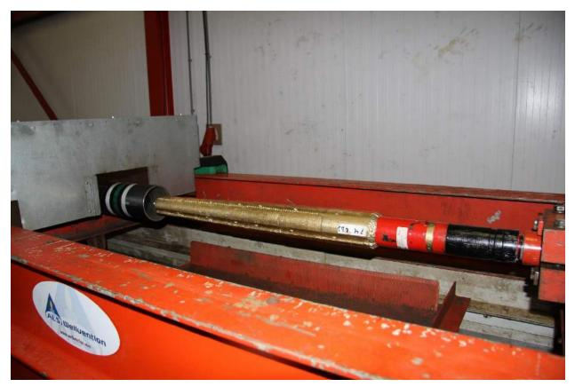
All mill tests have been performed with a 2-7/8" spirostar motor and a flowrate of 350 lpm.
