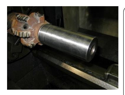
In July, 2009 QEP-LA asked us to convert a Hycalog Bicenter bit that they owned to a BCS by replacing the 5" pilot portion with a box thread. It was run between two concentric reamers (6") into a 6 1/2" drilled horizontal hole to open the hole to 7" using the 6" concentric reamers as a guide. It did ream the hole but almost got stuck several times.
