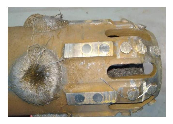
As of 10DEC19 we have slightly harder (#5) inserts being sent to the test site so the #3 inserts can be replaced for further testing.
