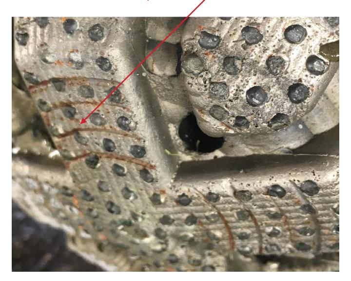
In this case we don't have a hydraulic cushion or the chip hold down that bits have, so the small grooves cut into the target (in steel) tend to form a chip that is not broken off easily so it will wear between diamond coverage. Notice the groove stops when coverage (number of blades) doubles.
