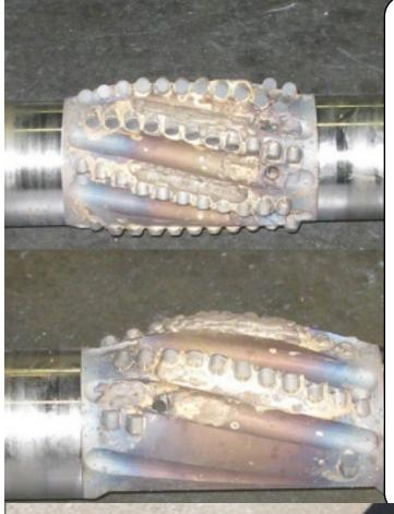
In August, 2009 Questar asked us at SBT to invent and build a BiCenter Sub (BCS) that would drift through 6" and open a 6 1/2" hole up to 7". Our BCS was NOT built like a bicenter drill bit which has cutter geometry facing down hole...ours was based on cutter geometry that would be free to cut sideways into the hole wall.
