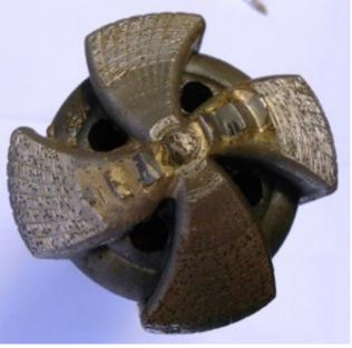
Second Run cut bottom part of Ball Valve in 4 hours WOB = 1500 to 2500 lbs (385 to 641 psi)
