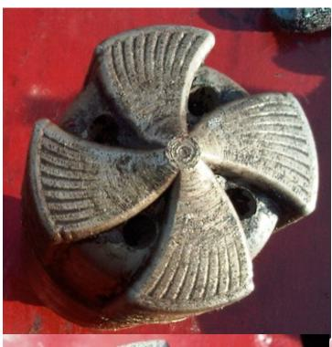
3.250" Standard MX mill at left failed to develop motor differential when starting to mill the flapper (wore tip)
