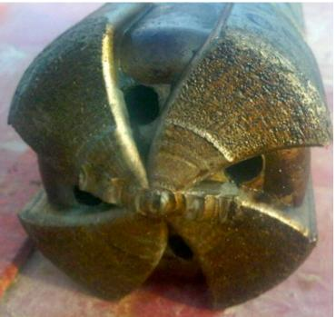
We ran the center carbide mill to mill the third flapper, it took 3 hours only to mill the flapper successfully and 1 hour for back reaming.
