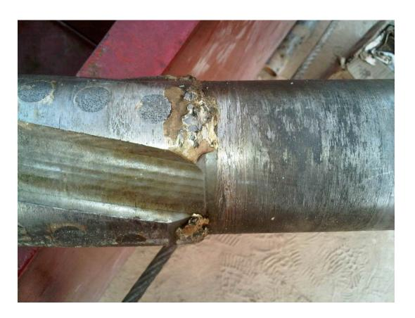
This is the diamond-impreg insert string reamer that has been run on 3 flappers on 4 trips.
