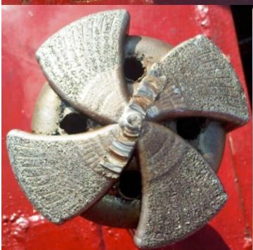
We ran the center carbide mill to mill the flapper, it took 3 hours only to mill the flapper successfully and 1 hour for back reaming, and we got a good differential during the milling operation.
