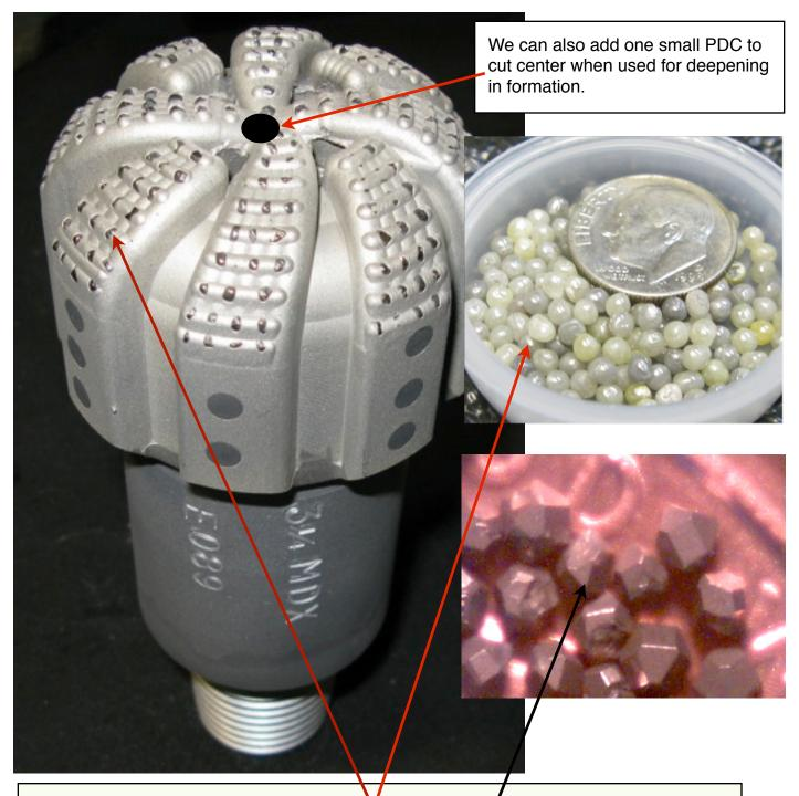
MDX Mills have two cutting structures. The primary one is natural diamonds set in ridges that are raised about .040" above the mill blades. The secondary cutting structure is titanium coated diamond grit (30-40 mesh) that is impregnated into the blades at about 20-25% by volume.
