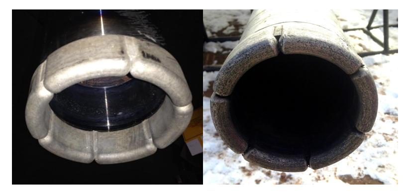
"Before and after burning over a 7" Hornet packer sitting at 60 degrees. The packer let go and started moving after 1-1/2 hours of drill time."
