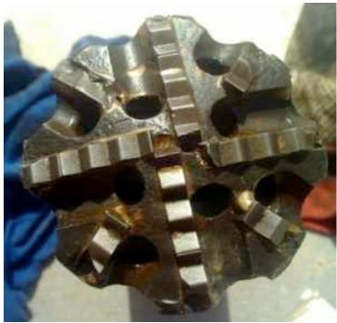
First Run used on motor/CT to drill five SLB aluminum "copperhead" plugs and "some other target".
