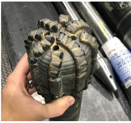
The first run was 2000 ft of 8.6 ppg cement (no plugs) drilling 2.5 to 3.0 ft/min controlled with granular cuttings
