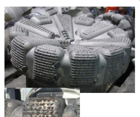
Serial Number X-289 had one rental run previous to this and was used to time drill at 1 fph for 7 hours to get a lip started...then 1" every 2 min (2.5 fph) and 1" every minute at 5 fph for remainder of 60 feet.
