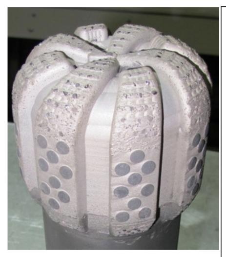
Based on previous runs of MD design we offered the MDX with updrill feature and diamond-impreg as backup for 1/4" depth into the blades.
