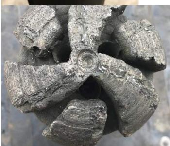
3 7/8" MX-C was ordered/ fabricated/and in the hole within 24 hrs and made a total of 190 feet to finish the job. As you can see the carbide inserts were not lost downhole even though they are completely shattered
