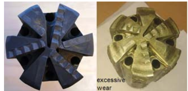
Before TT Turbodrill mill before and after first run
