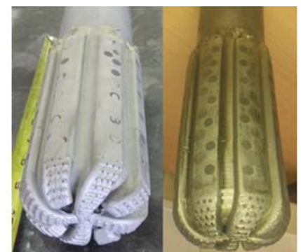
Before MDX Diamond mill before and after second run
