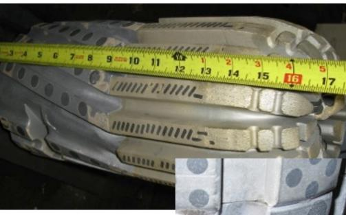
Plug Welds are made to join the 8620 sleeve with brazed-in inserts to the mandrel at the bit blank/weld area, at two places on the 4130 mandrel, and 360 degrees around the top sleeve/mandrel interface.
