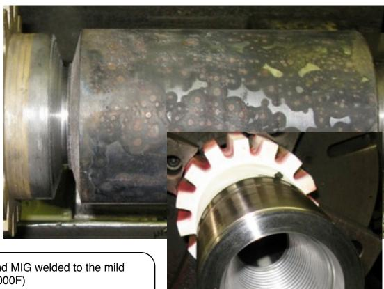
4130 HT Blank Mandrel is shrink-fit and MIG welded to the mild steel blank (pre-heat 600F/post heat 1000F) Slow Cooled in furnace heated to 1000F and turned off and let cool overnight.
