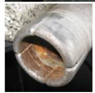
Target: 2 3/8" Cone-Buster Mill Stuck with loose carbide packed into the annulus just above it.
