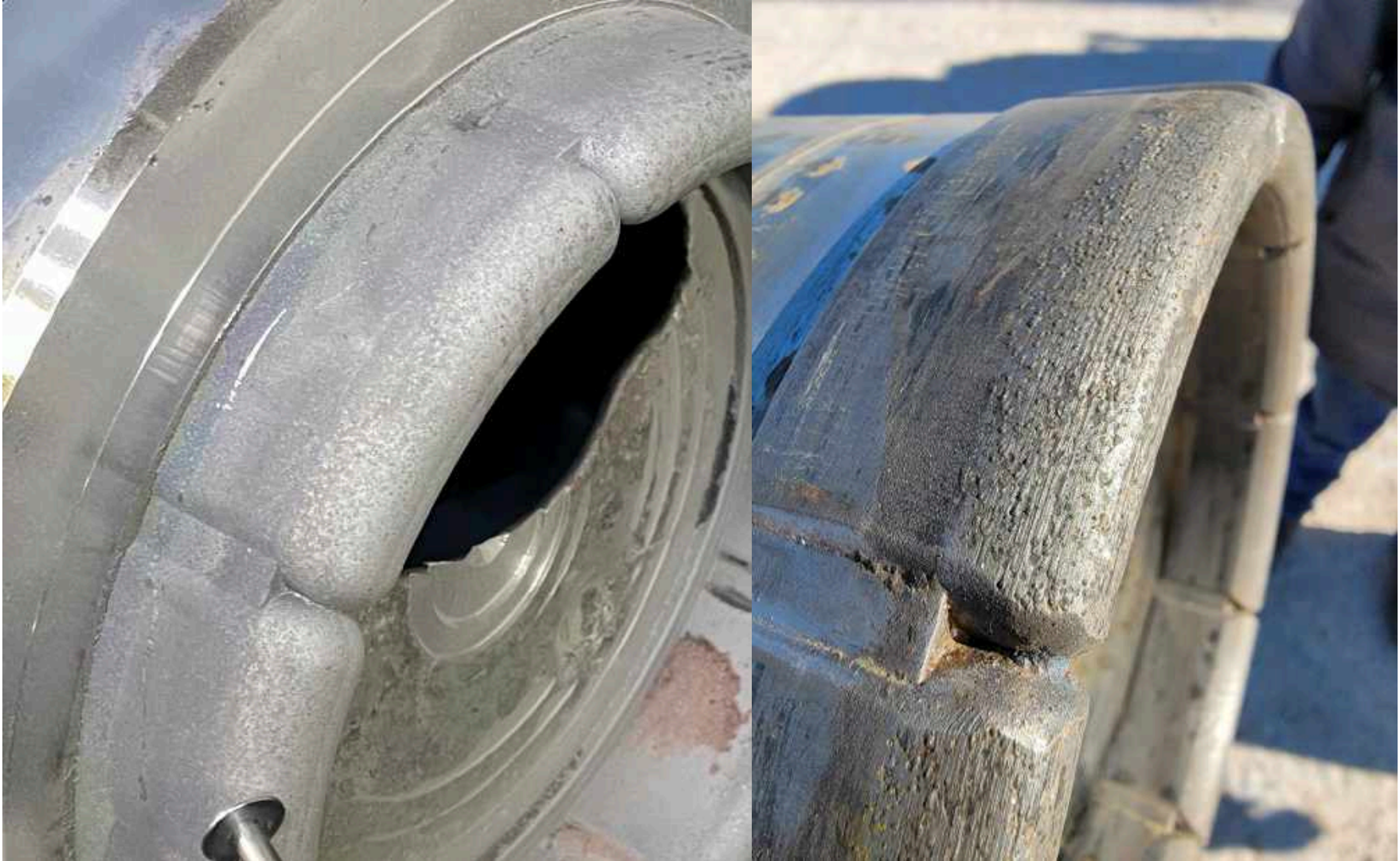
Top side of OD worn about .040" (no diamonds) Shoe Face worn about 1/8" (of 5/8") 36 ft / 64 hrs
