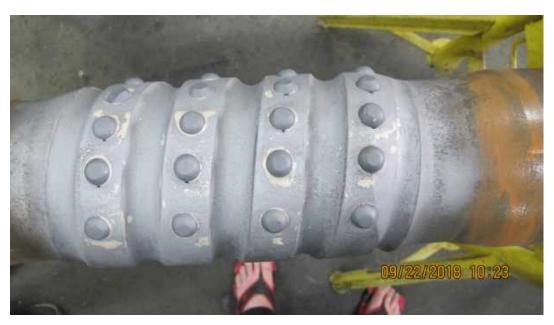
Eccentric Stabilizer after 14,000 ft reaming while drilling with no wear on the carbide dampeners because they do no work (no cutting...no reaming) since the drift diameter of the hole is already enlarged by the Reamer below it.
