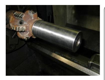
In July, 2009 QEP-LA asked us to convert a Hycalog Bicenter bit that they owned to a BCS by replacing the 5" pilot portion with a box thread. It was run between two concentric reamers (6") into a 6 1/2" drilled horizontal hole to open the hole to 7" using the 6" concentric reamers as a guide. It did ream the hole but almost got stuck several times.
