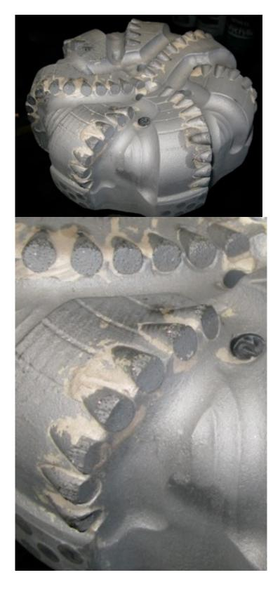
This bit type is intended for use in sidetracking operations when the target formation may damage PDC cutters or natural diamonds by impact loading. The KX-1 uses HPI (high pressure impreg) inserts that are mounted just like PDC cutters but the HPI's are much more impact resistant so they can have the cutting action of a PDC cutter but the abrasive resistance of diamondimpreg. They are brazed into the bit head so they can be refit after dulling.
