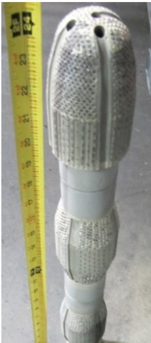
Matrix Body / Exposed Spherical Diamonds in both the lead mill (Crayola) and Follow Mills. These are about 8" each and can be made to stack as shown at left with a lead and two follow or below as either one lead and one follow or two follows.
