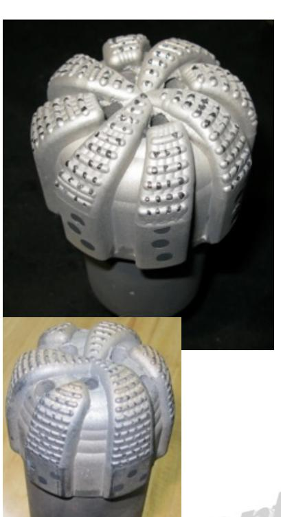
MDX Mills were developed specifically for hard scale milling but have been used with good results in other hard applications.
