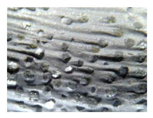
Grit sized synthetic diamonds are titanium coated and then encapsulated in a blend of Tungsten/Tungsten Carbide powders. This slurry can then be packed into mold details to form almost any shape in a bit, mill, or shoe face.
