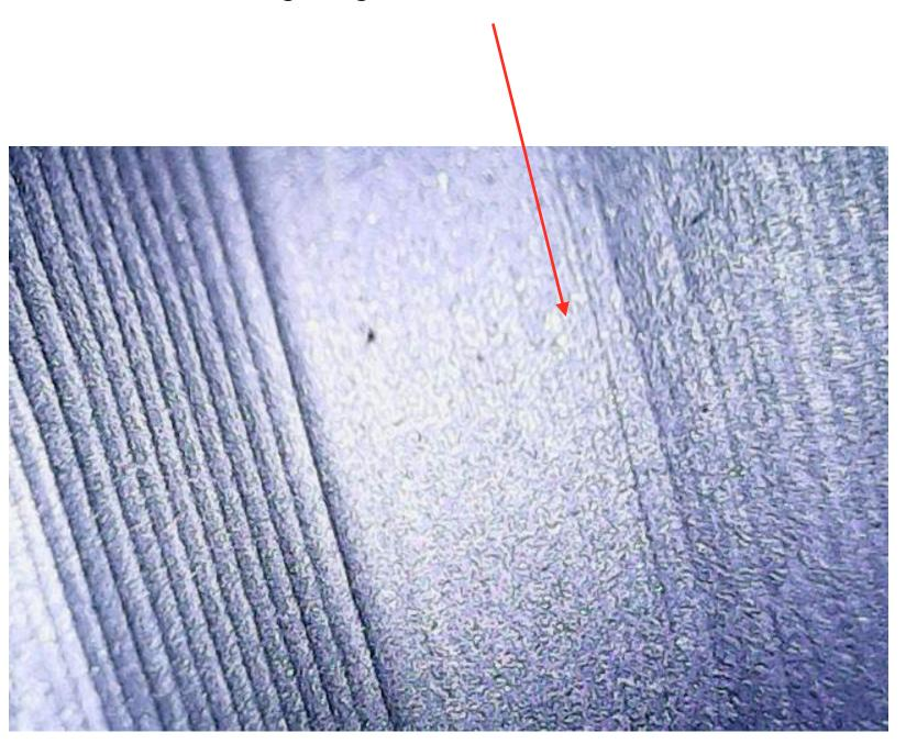
Yet when a magnetic field is applied and magnetic particles are applied the media will gather at the SEAM. This is NOT a crack.
