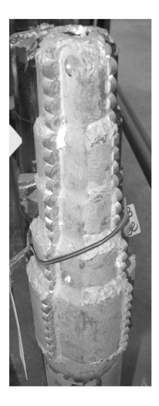
Carbide Step Mills (Stage Mills) can be custom fabricated to the client's desired shape and cut per stage using round, square, hex, or octagonal inserts.
