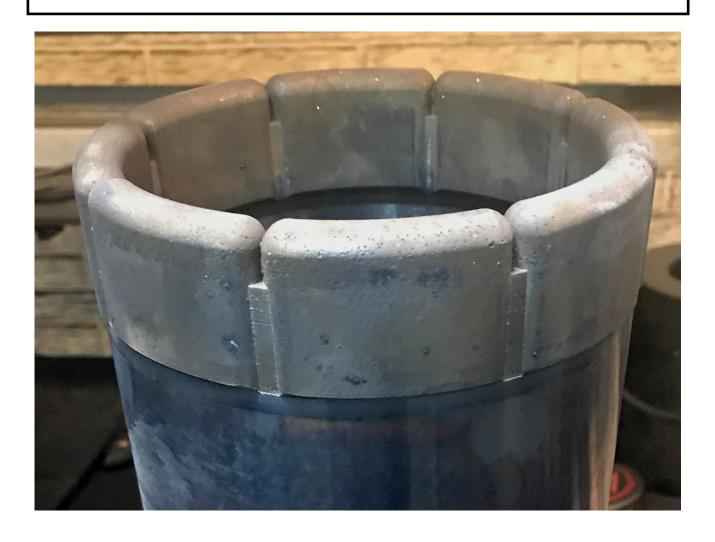
Our HYBRID XDSC adds 3/8" round carbide chip breaker inserts to each leading edge to take advantage of softer materials such as seal components of packers, mild steel, cement, dehydrated mud.
