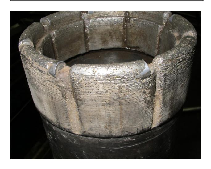
Our HYBRID XDSS adds small sharp Star-Bide carbide inserts that are slightly exposed to help cut certain alloys that work harden such as 13 chrome, 9 chrome, inconel 718, and incology 925
