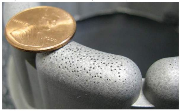
The shoe head has a valid cutting structure until this 1/2" is used up. This type of cutting structure has been used to cut hard steel, case hard steel, carbide, 13 chrome, inconel, as well as many softer components.
