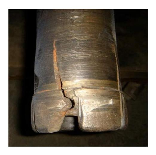
This XDS shoe was used on jointed pipe to burn over one plug with carbide slip buttons and then was used without rotating to push downward on the fish with 20,000 pounds which belled the shoe head. The internal failsafe mechanical locking of the worked so that only a small amount was lost downhole. XDS shoes are not intended to have such high forces transferred through them...especially when not rotating.
