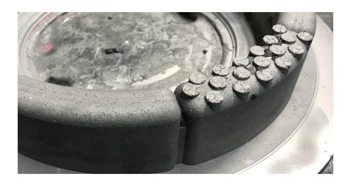
Your XDSS shoe has an added feature of having 33 exposed plots in four of the eight "pods". These are intended to give you an initial low area to penetrate (est 900 to 1800 lbs) so if your target is softer that expected you can take advantage with this small area. There are two 1/8" star-bide pellets in each plot. If harder target is cut they should wear down to the diamond-impreg without much effort. From that point you have 1/2" of diamond grit that is about 30% of the volume of the shoe head.
