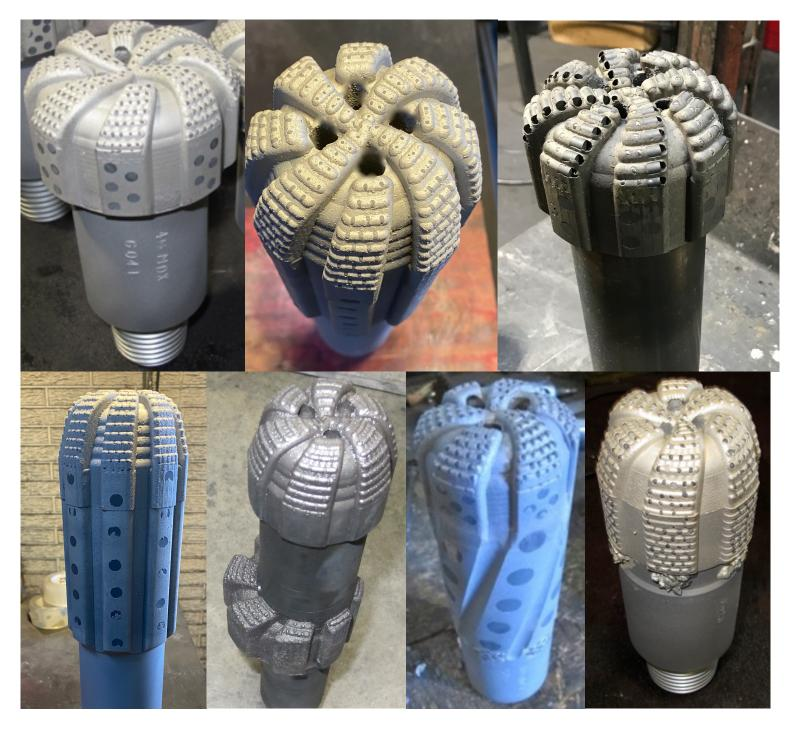
MDX Mills can be custom fabricated with several optional features. Spherical Diamonds are set in raised ridges to resist impact fracture . Diamond Grit is impregnated 1/4" deep into the face matrix to resist undercutting. Used primarily to cut hard scales, MDX Mills have been used on several other applications with good results...compacted frac sand, composite plugs, ball seats and others.
