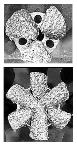
SJ-3 mills have three blades set with coarse carbide chips.
