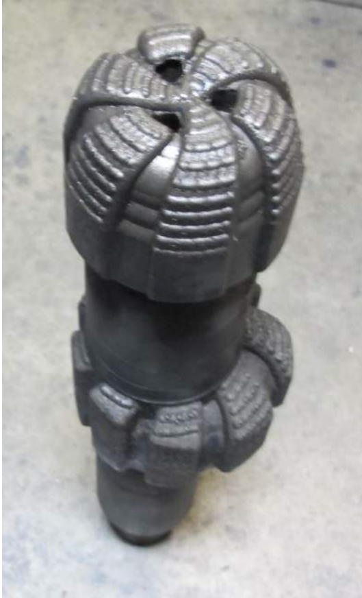
MDX-BC Matrix Body with Spherical Diamonds backed with 30-40 mesh diamond impreg
