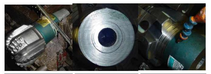
A Smith Rotary Drill Bit has its top sub sawn off just above the weld line.
