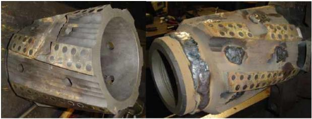
The sleeve stabilizer is cut from billet steel, milled, drilled, assembled, brazed and ground true, then it is slip fit onto the mandrel...aligned with your bit gage, pre-heated to 550-600F, and 7018 MIG welded in the plugs and circumference.
