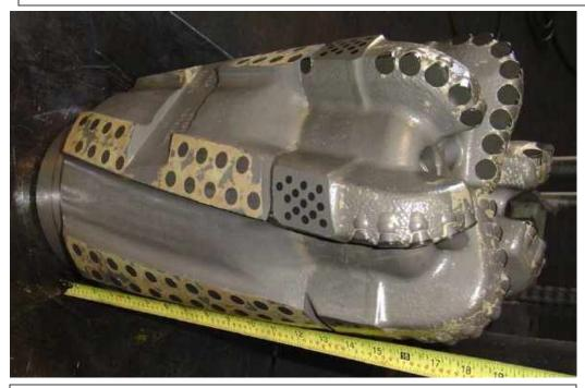
There is a net reduction in annular area of about 30% from the bit to the sleeve stabilizer.
