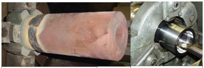
A 4130 HT Mandrel is made to match the original OD of your bit shank to keep the originaldesign strength at your bit matrix to mild steel blank interface. We do not alter your original bit structure.
