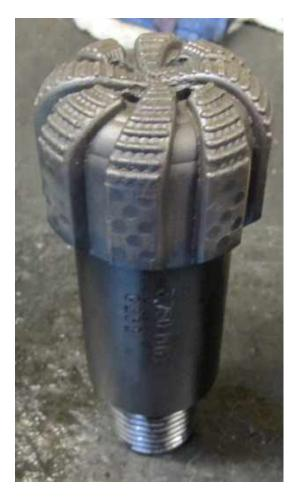
MDX mills have a primary cutter geometry of spherical diamonds set in raised ridges and a secondary cutting geometry of 30-40 mesh diamond grit that is impregnated into the first 1/4" of mill face.
