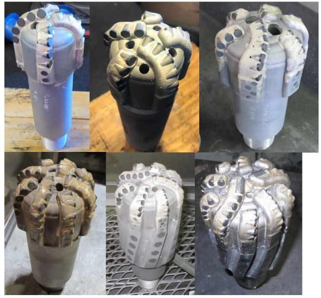
MZ Matrix/PDC mills are purpose built for Thru-Tubing applications to drill long intervals of hard cement, hard scales, frac plug drill outs, and some formations.
