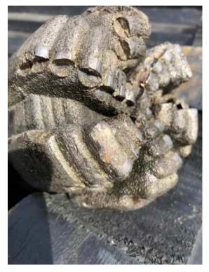
These mills have a primary cutting geometry of normal diamond impreg and a Hybrid cutting structure of carbide inserts
