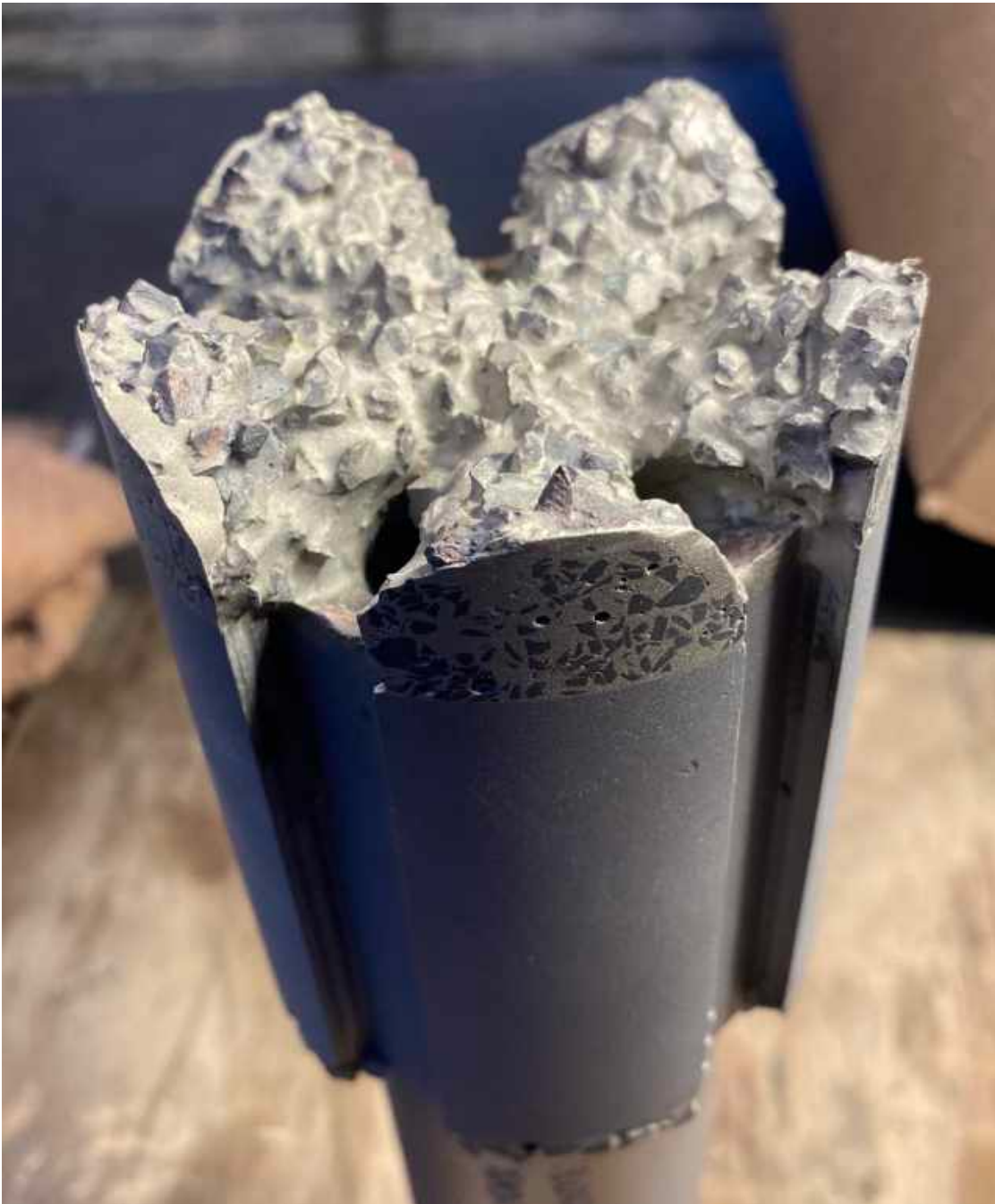
SJ-Conical Medium WC Chips
