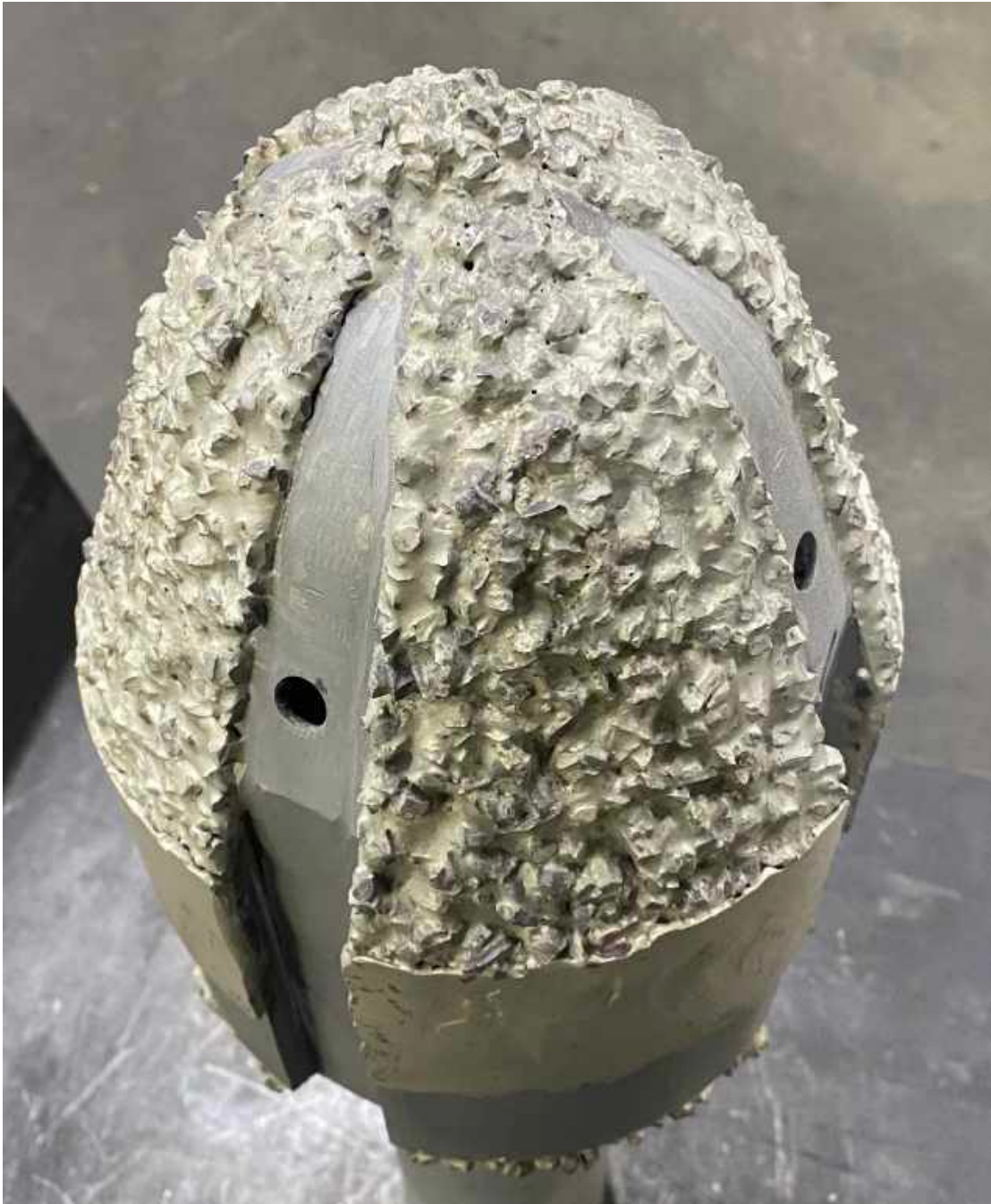
SJT Slight Taper 30 Deg / Medium WC Chips Updrill
